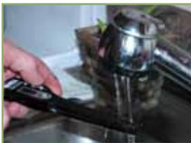
1. To also ensure efficiency, use a digital thermometer to check the temperature of the hot water. Turn a faucet on hot and after maximum heating has taken place, take a reading.
