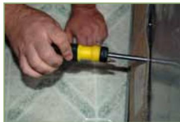
3. If necessary, use the screwdriver to remove the back cover or kick plate to access the coils.
