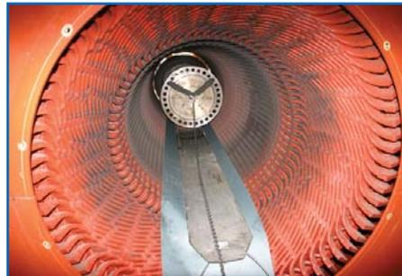
An inside look at a stator with the turbine shaft coming in which connects to a rotor.
